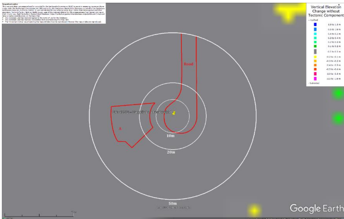
Figure 27: Ground surface subsidence without tectonic component for Jun 2011 Earthquake according to the LiDAR DEM.
