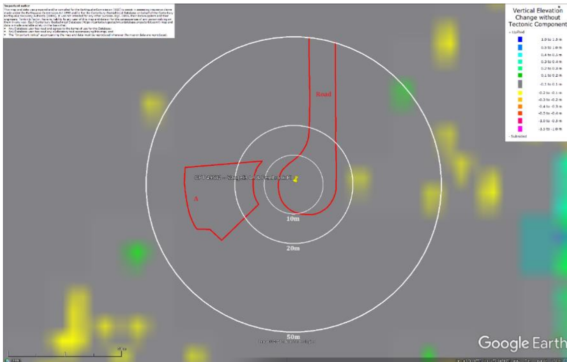
Figure 26: Ground surface subsidence without tectonic component for Feb 2011 Earthquake according to the LiDAR DEM.
